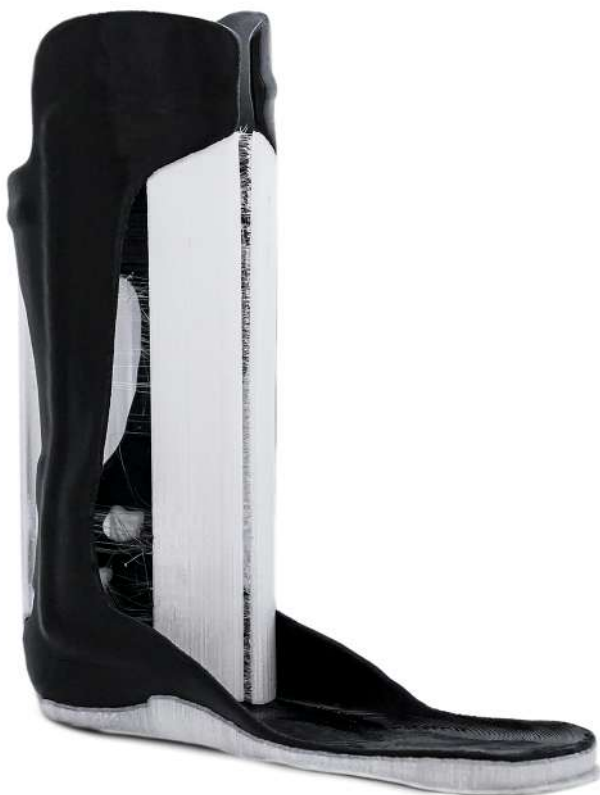
Figure 3: Extrusion-based 3D printed leg splint (black) made from PP. For the production ‘P-filament 721 black’ and the specially for PP developed breakaway support material ‘P-support 279’ (white) were used.
